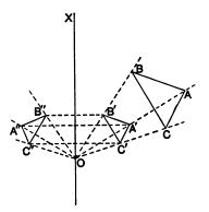
It is obvious that the triangle A''B''C'' is inversely similar to the triangle ABC. It is also evident from the figure that the triangles OB''C'', OC''A'', OA''B'' are inversely similar to the triangles OBC, OCA, OAB; that the angles AOA'', BOB'', COC''are bisected by the line OX; and that
